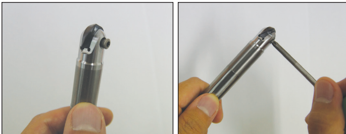
▲ Slide the insert into the slot of the holder Tighten the screw using anti-seize compound
